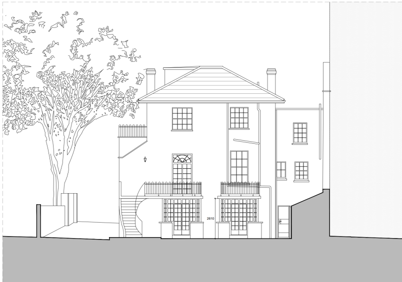
Existing Rear Elevation 1:100 @ A3
